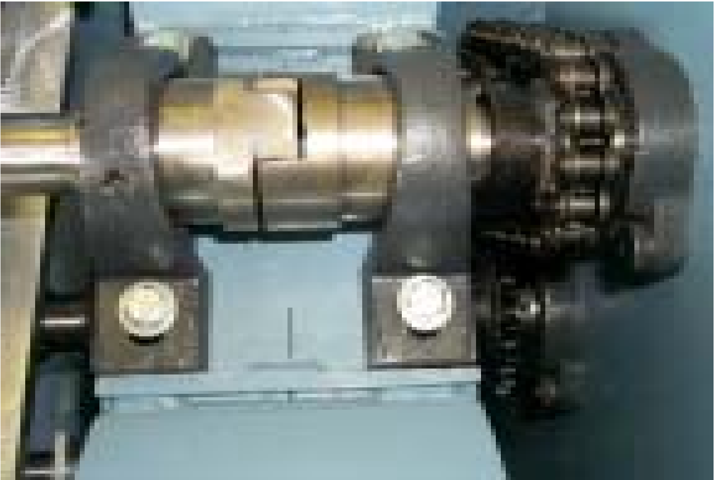
Figure #3 View of proper drive shaft joint orientation for removing a shaft
