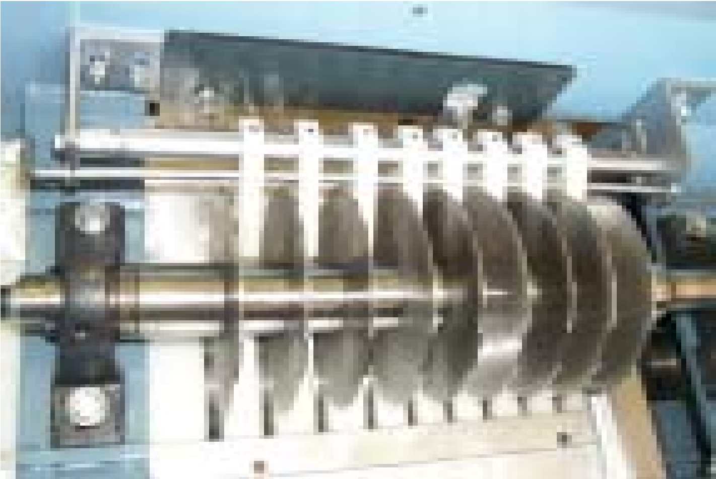
Figure #5 showing overhead view of table slot spacers
