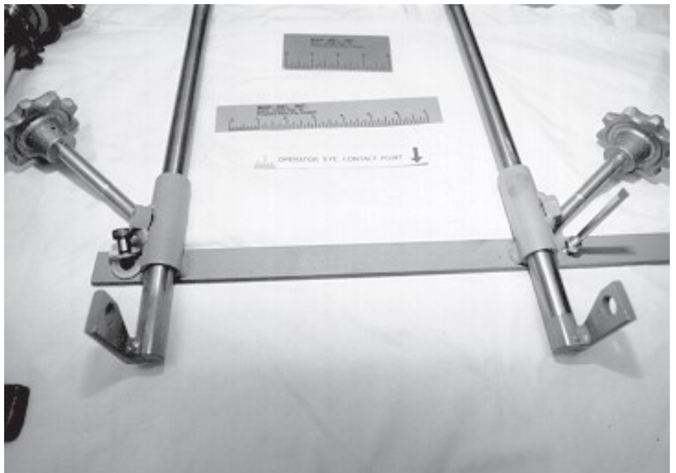
Double Slide Fence Assembly
